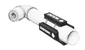
The Power Cells should be secured firmly around the pipe using the self-locking plastic straps provided. The Power Cells should be orientated with the fluid flow direction as per arrows on the units.
