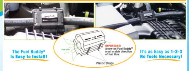
STEP 1 Locate accessible area on fuel line after filter and before combustion area (carburetor). Situate unit closest to combustion point.
