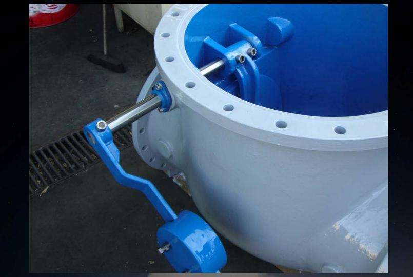
Internal area was coated with minimum 600 microns CeramAlloy CL+AC Outside surface with minimum 350 microns CHEMCLAD SC
